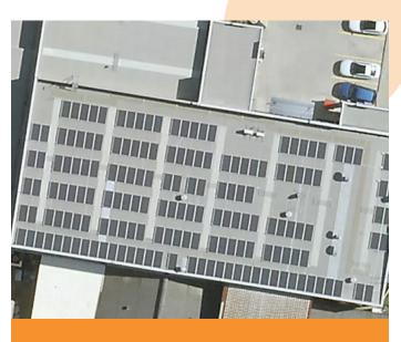
System Size: 62kW Location: Fairfield East, NSW Panels: 168 X Trina 365W Inverter: 2x Solaredge 27.6kW Additional: SolarEdge DC Optimizers (P700)
